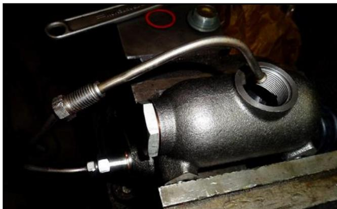
The image is a new master cylinder being held tightly in a vise. You will notice that the fitting at the bottom rear of the cylinder has been installed onto the new master cylinder. SEE THE BOTTOM LEFT OF THE MASTER CYLINDER. This fitting is about 1" long and has a male thread which screws into the master cylinder on one side and has a female tread on the other side where the brake line from the three way fitting on the frame rail screws into.
