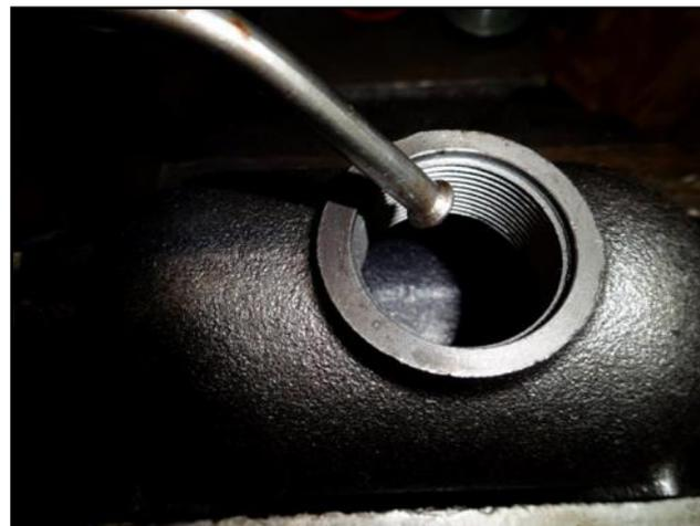
This photo shows where the other end of the temp. brake line should end up. What you've just done is create a loop of brake fluid that goes out of the master cylinder and back into the filler inlet. You are not using any additional fluid.
